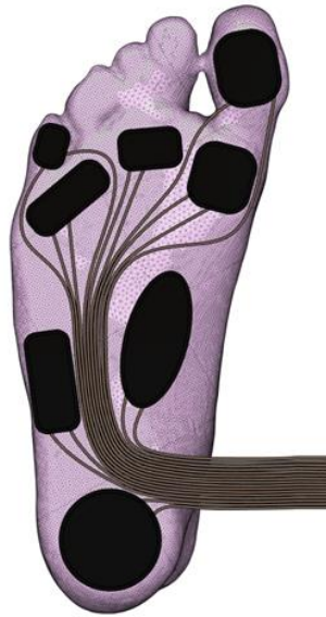
Figure 2: Design of the eight-sensor insole
